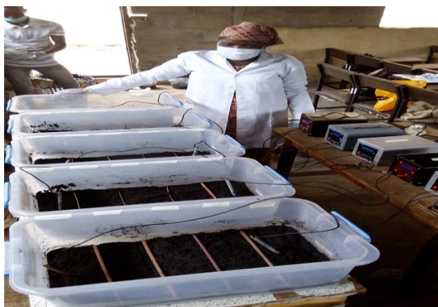
Figure 1: Schematic Diagram of Electrokinetic Reactor
